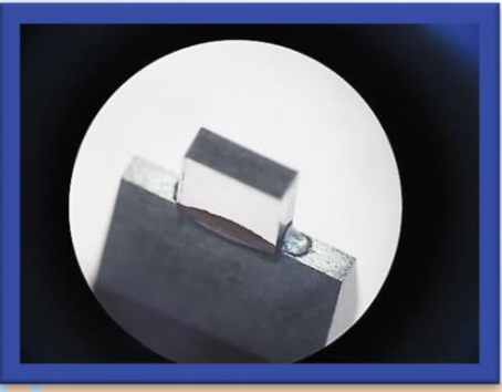
⑦ Mounting To install the stone on holder.
