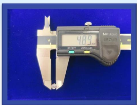
② Measurement 1 The length of stone is 4.89mm.
